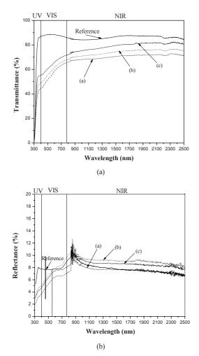
Fig. 5. Triboadhesion test results on a soda-lime glass sample coated with iron oxide by triboadhesion: a) Optical transmittance and b) reflectance. The terms UV, VIS and NIR represent the Ultra Violet, Visible and Near Infrared spectral radiation regions.
