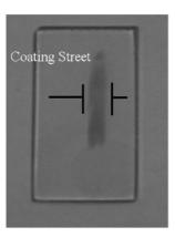
Fig. 3. Soda-lime glass sample coated with iron oxide by triboadhesion.
