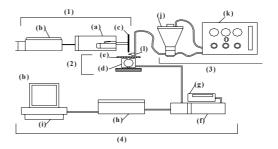
Fig. 1. Deposition process: 1. Rotating wheel system: (a) high speed motor, (b) velocity control, (c) mop; 2. Force measurement system: (d) ring type load cell, (e) base; 3. Feeding system: (j) particles container, (k) pneumatic control system, (l) nozzle; 4. Data acquisition system: (f) amplifier, (g) volt-meter, (h) signal analyzer, and (i) PC [6].
